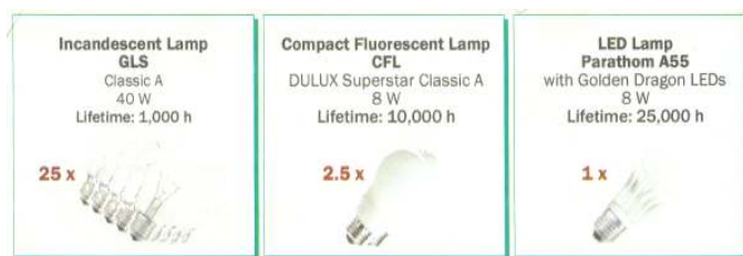
A 40W incandescent lamp, an 8W compact fluorescent lamp and an 8W LED lamp with six LEDs were used in the LCA.
