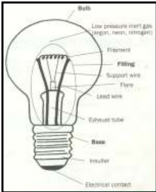
Various parts of an incandescent bulb.
